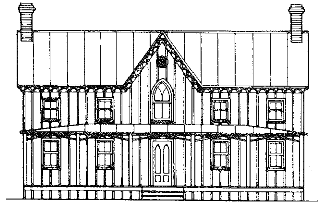
Figure 16.17 Gothic Central Passage (Board-and-Batten Siding).
